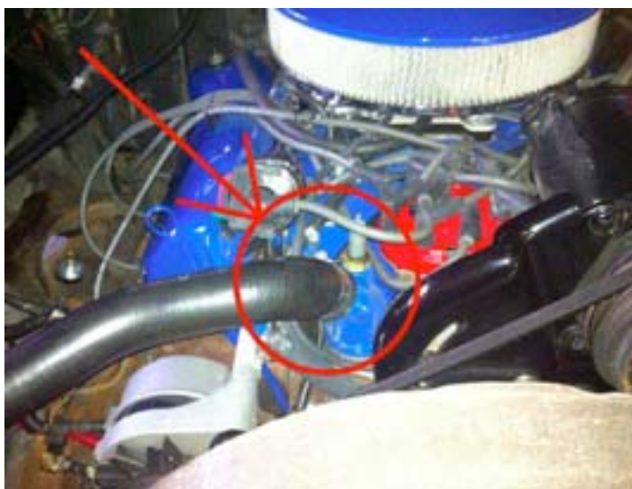
This hose slipped off with the clamp
