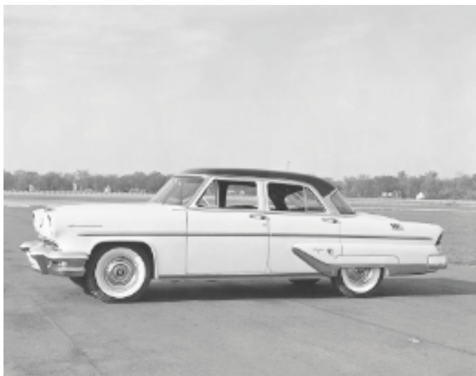
The 1955 Lincoln Capri featured a flat windshield despite the popularity of the wrapped windshield.
