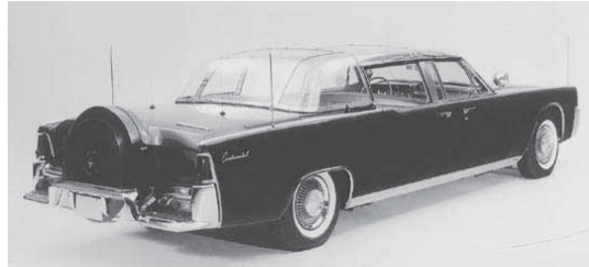
5 After JFK's assassination, the X-100 Lincoln was rebuilt as a closed limousine with a transparent top. It's shown here with the 1962 front grille and 1956 Lincoln Premier wheel covers.
