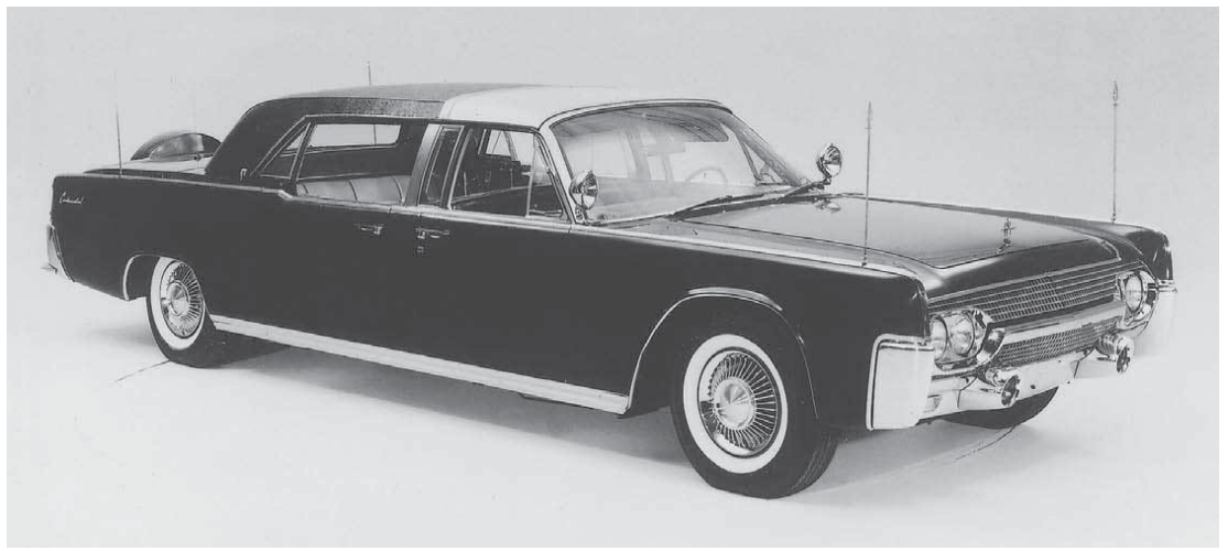
5 Shown in its original form when first delivered to the White House, the X-100 Lincoln parade car has the 1961 grille, Continental Mark II wheel covers and the Plexiglas top in place with the protective cover over the rear portion of the passenger compartment.
