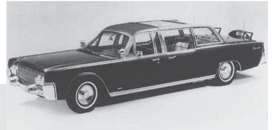
5 After JFK's assassination, the X-100 Lincoln was rebuilt as a closed limousine with a transparent top. It's shown here with the 1962 front grille and 1956 Lincoln Premier wheel covers.
